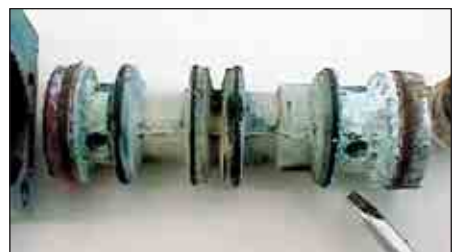
Contaminants corrode and damage air-operated equipment
